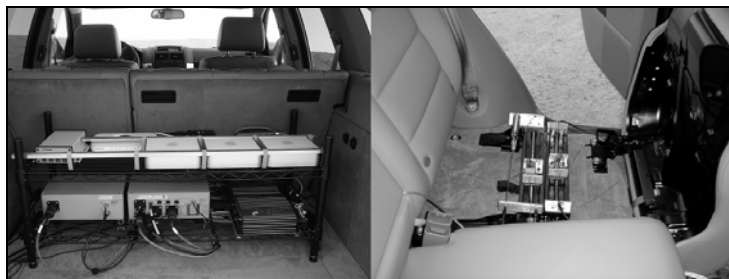
Look who's driving: The VW Touareg was chosen to provide a stable, climate controlled environment for Dora's sensitive electronic equipment, including the three Mac Minis and drive control actuators pictured above.
